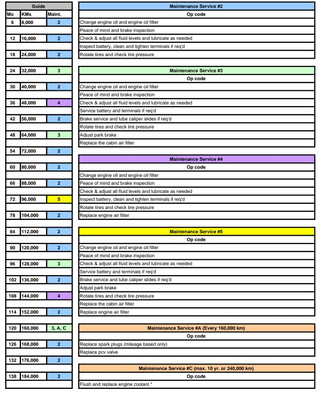
Guide is based on Fiat Chrysler Canada factory required maintenance. Change Engine Oil & Filter when prompted by Indicator system. Under no circumstances should oil change interval exceed 16,000 km or 12 months, whichever comes first. Other services: \* Not to exceed 120 months or 240,000 km.
