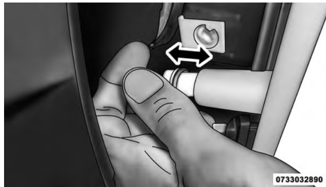
Front Side Marker Lamp Bulb Removal
